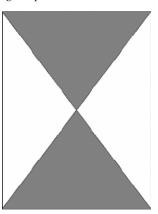
The lamps or plates must be on the same height above buffer on the transversal axis.
