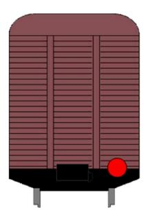
The reflective disc shall have a diameter of 185 mm with a red circle diameter of 140 mm. Where justified by operating practices, the reflective disc may be replaced with one reflective plate in compliance with Appendix E to TSI WAG.
